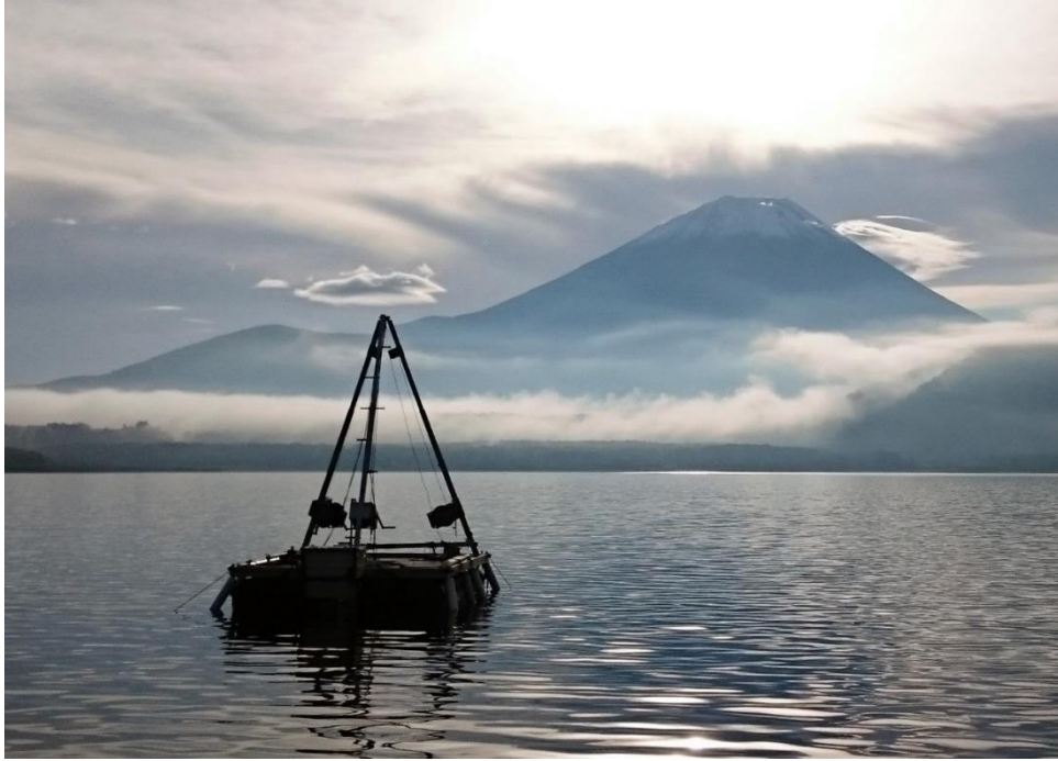
Figure 1: Coring platform in Lake Motosu. The core sampler is lowered from the triangular derrick.
