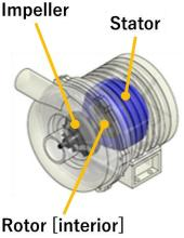
Figure 2. Ultra high-speed motor example
