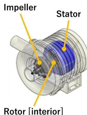
Figure 2. Ultra high-speed motor example
