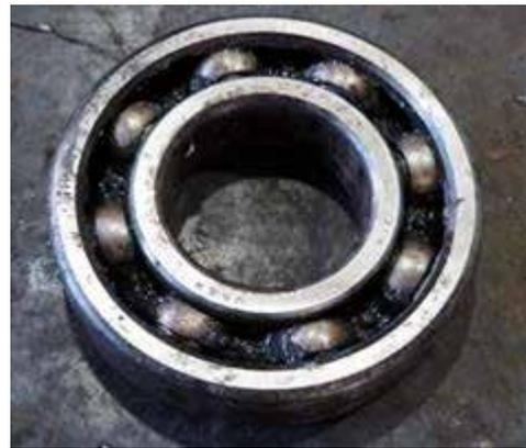
Figure 2. Failure (eroded by pollution)
