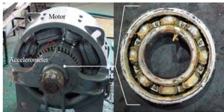
Fig 2. Vibration data collecting
